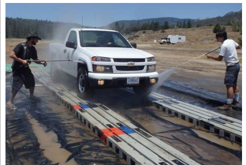
For weed wash stations, raised tracks are important to keep vehicles from driving through weed seeds shed from other vehicles. Water is captured, filtered, and re-used. Photo: Joanna Clines.
