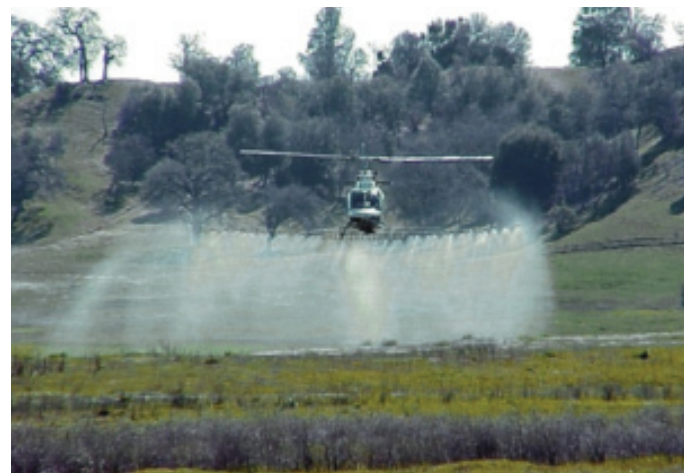
GPS-guided helicopter application. A helicopter with on-board GPS was used to accurately apply clopyralid in a long-term management study at Fort Hunter Liggett. (Photo: A. Hazebrook)
